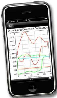
The LRP® system incorporates Unico's patented SRP sucker-rod pump control software to optimize production while protecting the pumping system. Sophisticated variable-speed control achieves motion profiles that are impossible through mechanical means.
