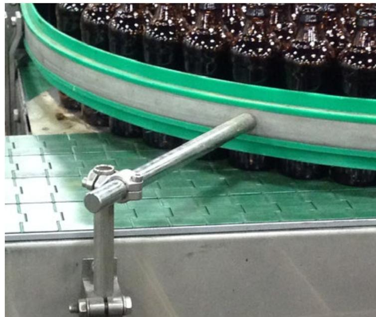
*System Plast New Generation (NG) chain is made of a proprietary high-performance thermoplastic with a low coefficient of friction. The flat conveyor chain lowers power consumption and noise, and increases chain life up to 50 percent in some applications.*
