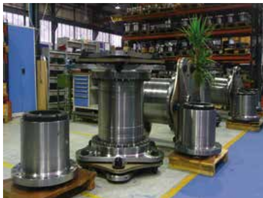
Jaure JHC-F-320 in combination with Lamidisc1300-6
