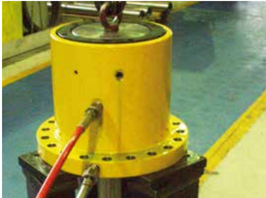
JHC-F-190 assembly test in house
