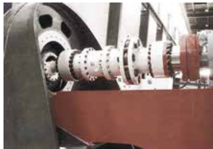
LAMIDISC® Safety coupling on test bench Incl. SAFESET® (SAFESET® from VOITH TURBO)
