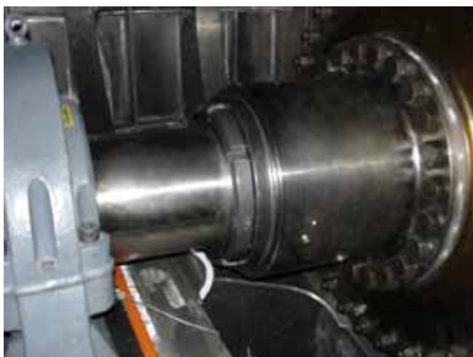
Jaure JHC-F-240 for Water Jet Drive
