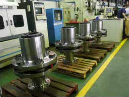
Jaure JHC-F-230 integrated with Lamidisc 730-6
