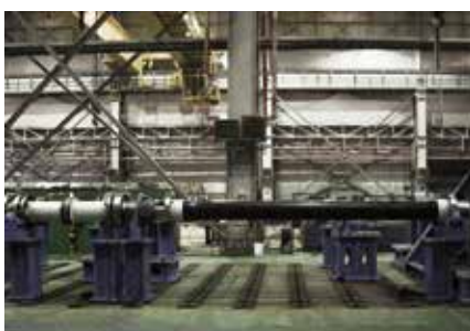
Carbon Fibre Shaft combined with LAMIDISC® coupling.
