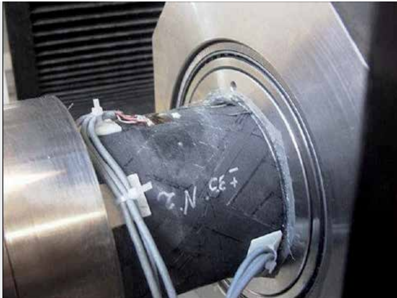
Testing of interlaminar and intralaminar shear strength
