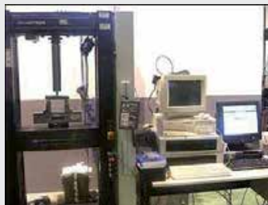
Testing of interlaminar and intralaminar shear strength
